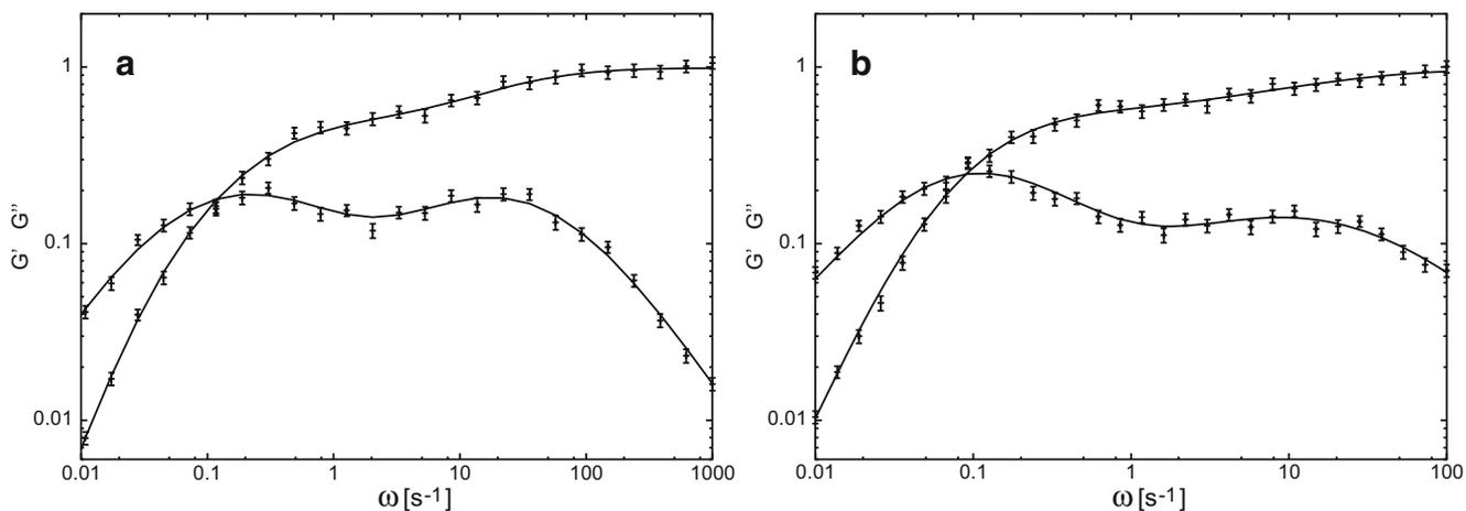
**Fig. 1** **a** Error bars simulated data from example a added 8% Gaussian noise. Full line typical fit of data. **b** Error bars simulated data from example b added 8% Gaussian noise. Full line typical fit of data
